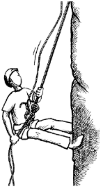
hand and body position during abseiling
