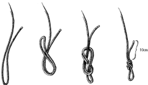
figure of eight knot in safety rope
