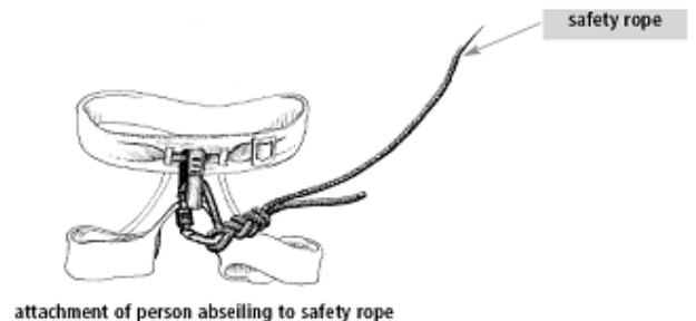
attachment of person abseiling to safety rope
